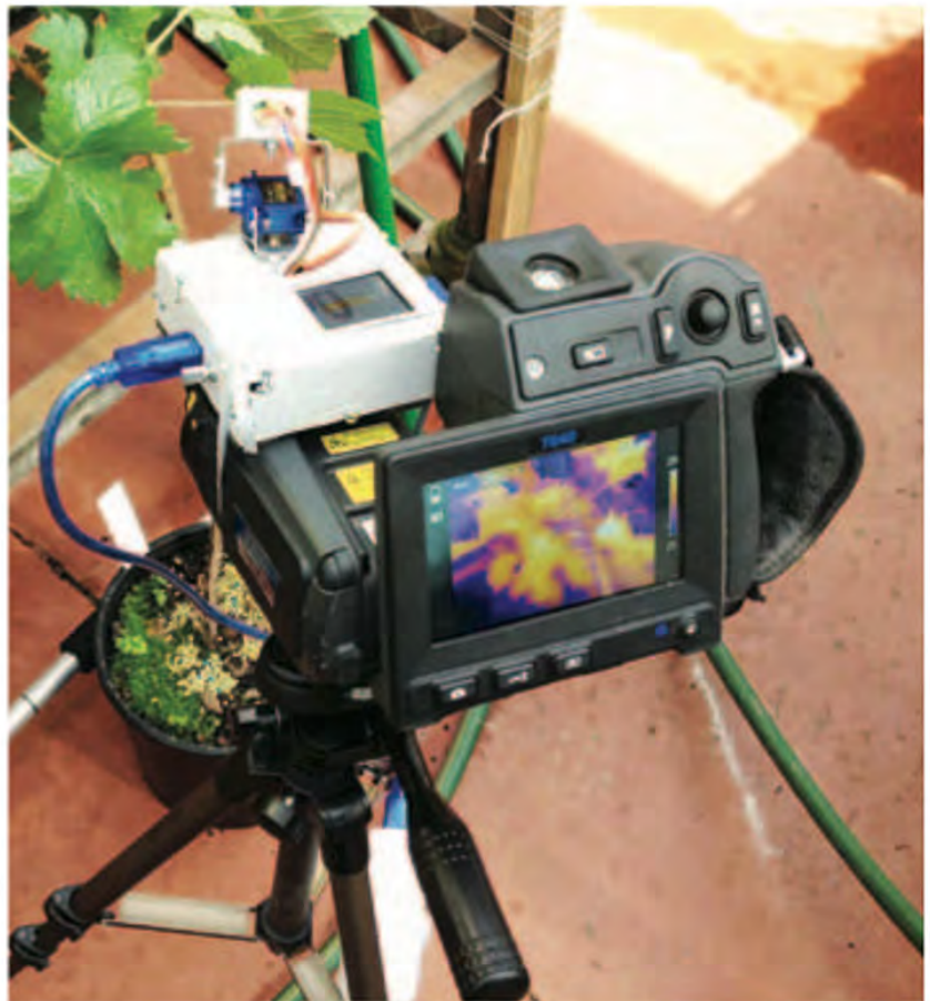
Say cheese: Infrared camera taking a thermal image from grapevines in the glasshouse. On top of the camera is an IR scanner with a 1 per cent cost compared to the thermal camera which is currently under testing by the VoF (Australia - Chile).
